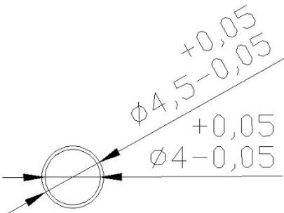
Figure 9-3 Input terminal size
