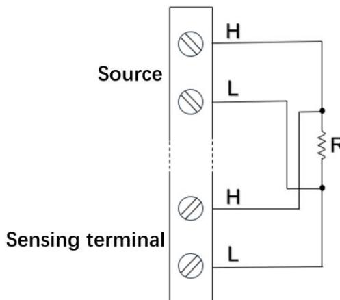
Figure 6-27 4-wire resistor
