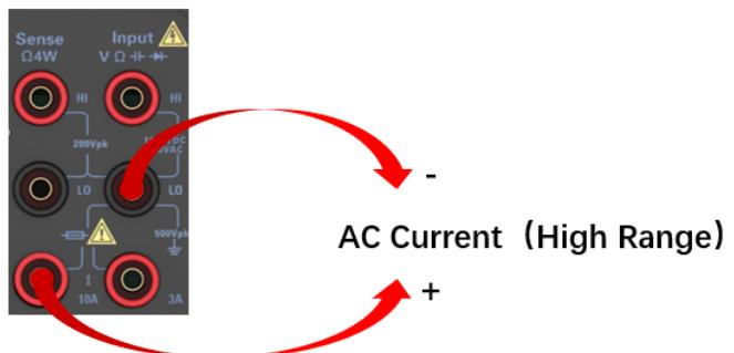
Figure 9-17 AC current (large range) connection diagram
