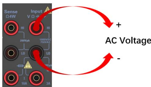
Figure 9-37 Frequency/Cycle connection diagram
