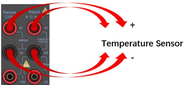
Figure 9-26 4-wire temperature connection diagram
