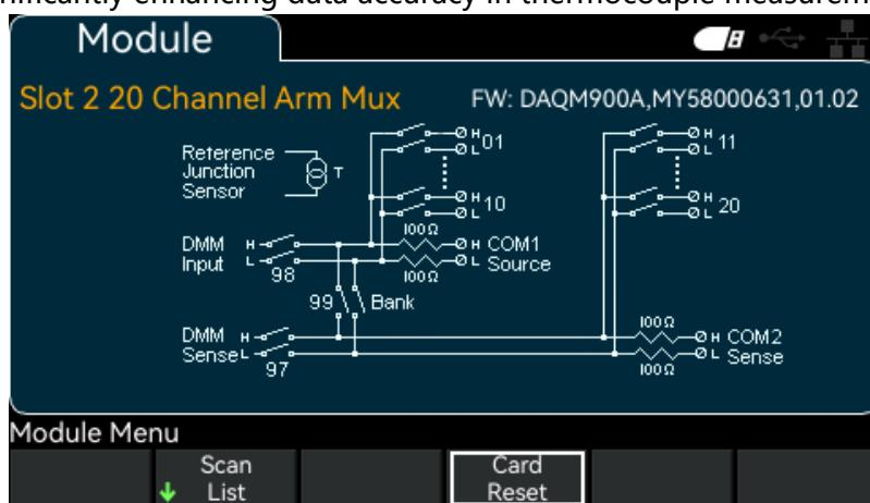
Figure 8-1 DAQM4000A multiplexing module
