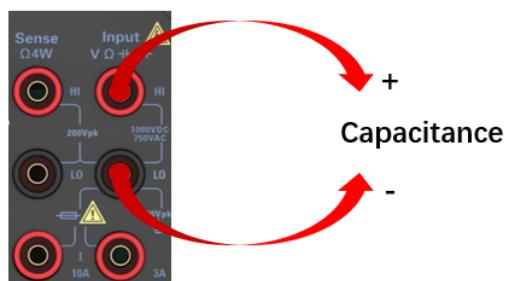
Figure 9-30 Capacitor connection diagram
