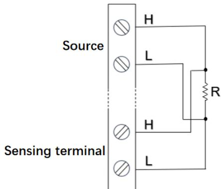
Figure 6-14 4-Wire thermistor
