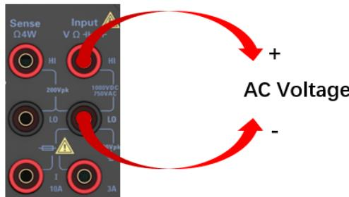
Figure 9-8 AC voltage connection diagram
