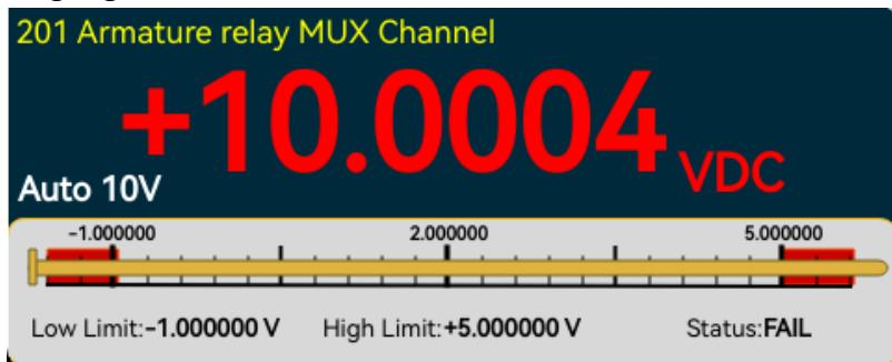
Figure 6-50 Bar meter-Alarm
