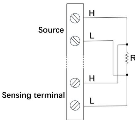
Figure 6-21 4-Wire direct strain
