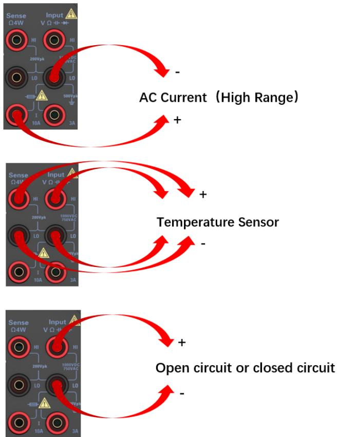
Figure 9-2 Measurement connection diagram
