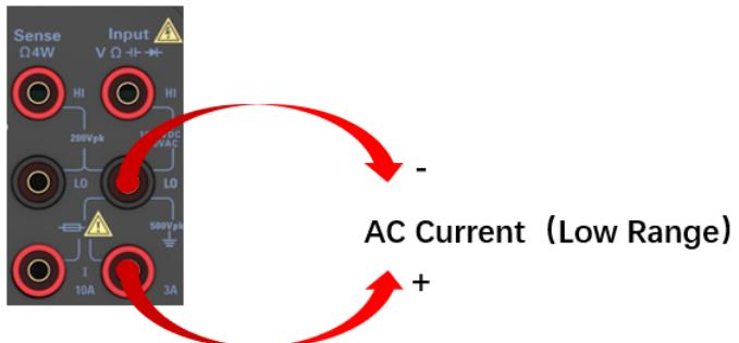
Figure 9-16 AC current (small range) connection diagram
