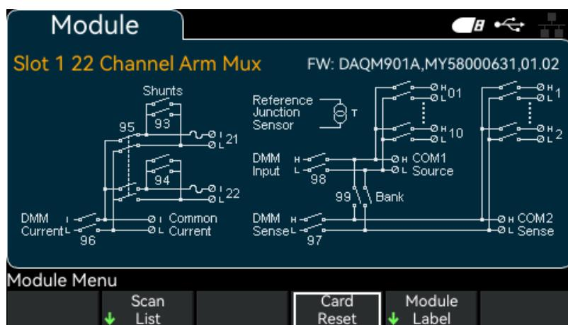
Figure 8-2 DAQM4001A multiplexing module
