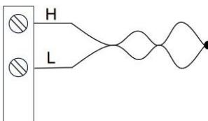
Figure 6-12 Thermocouple wiring diagram
