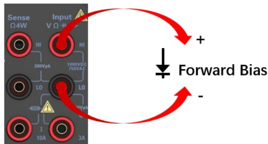
Figure 9-33 Diode connection diagram
