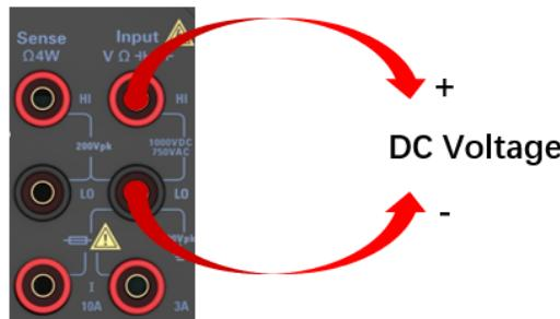
Figure 9-4 DC voltage connection diagram
