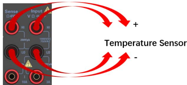
Figure 9-25 2-wire temperature connection diagram
