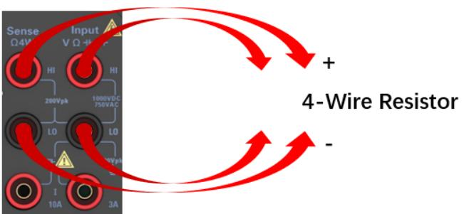
Figure 9-22 4-wire resistance connection diagram
