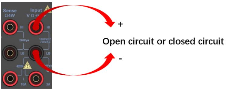
Figure 9-35 Continuity testing connection
