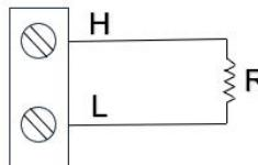
Figure 6-20 2-Wire direct strain
