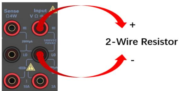
Figure 9-21 2-wire resistance connection diagram
