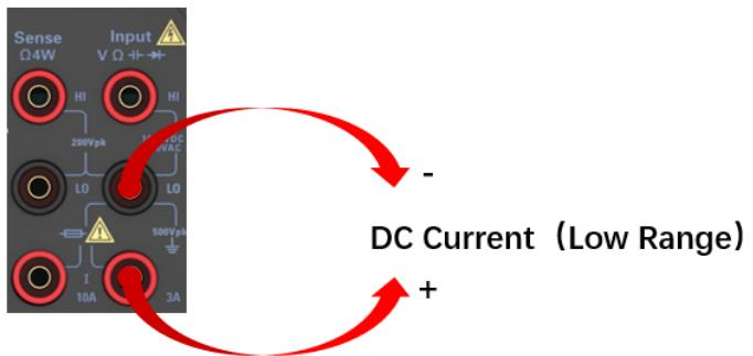
Figure 9-12 DC current (small range) connection diagram
