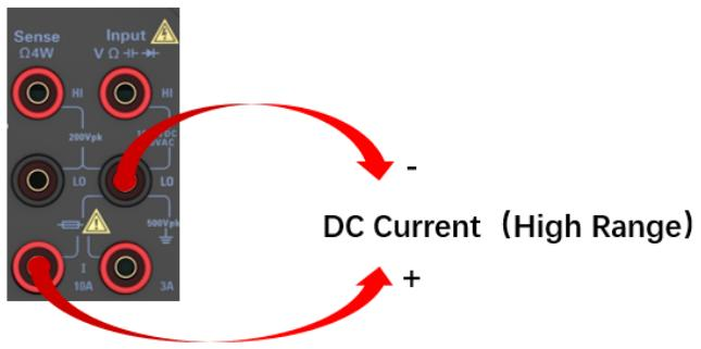
Figure 9-13 DC current (large range) connection diagram
