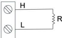
Figure 6-13 2-Wire thermistor
